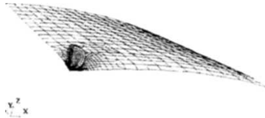
Fig. 3 Finite element mesh used for the R1500 \times R1000 , 600 mm panel
